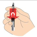
The bits can be inserted in all adapters with magnetic and will be locked into the adapters automatically.
