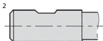
DIN 1835 B/DIN 6535 HB up to \varnothing 20 mm
