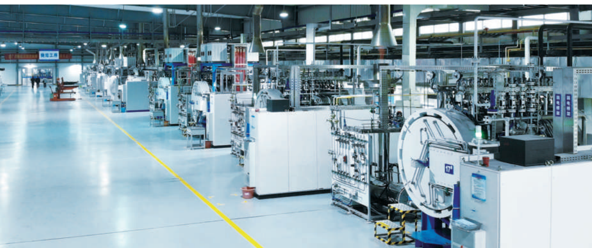
Sintering of inserts
