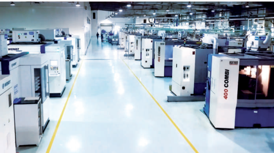
Grinding of inserts
